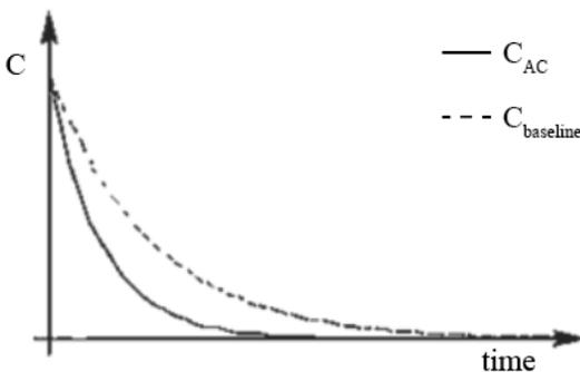
Figure 1. Concentration of pollutant as a function of time with and without an AC operating. <sup>8</sup>
