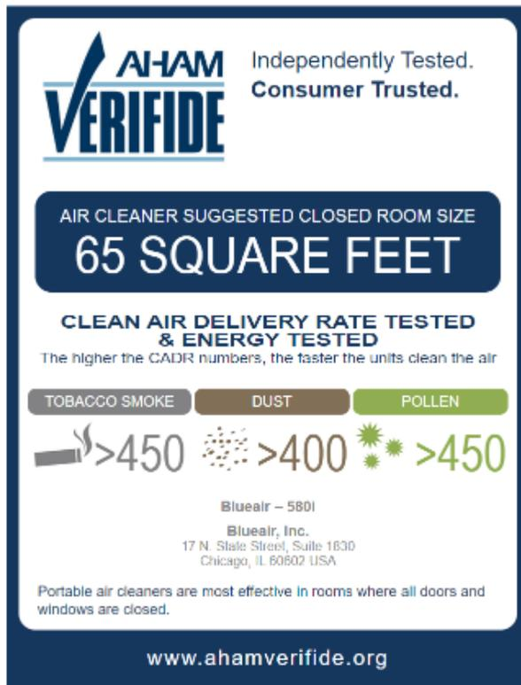
Figure 2. AHAM Verifide certificate showing the CADR values and room area for a Blueair – 580i air cleaner. (Note: the authors believe that there is an error on the certificates from the
