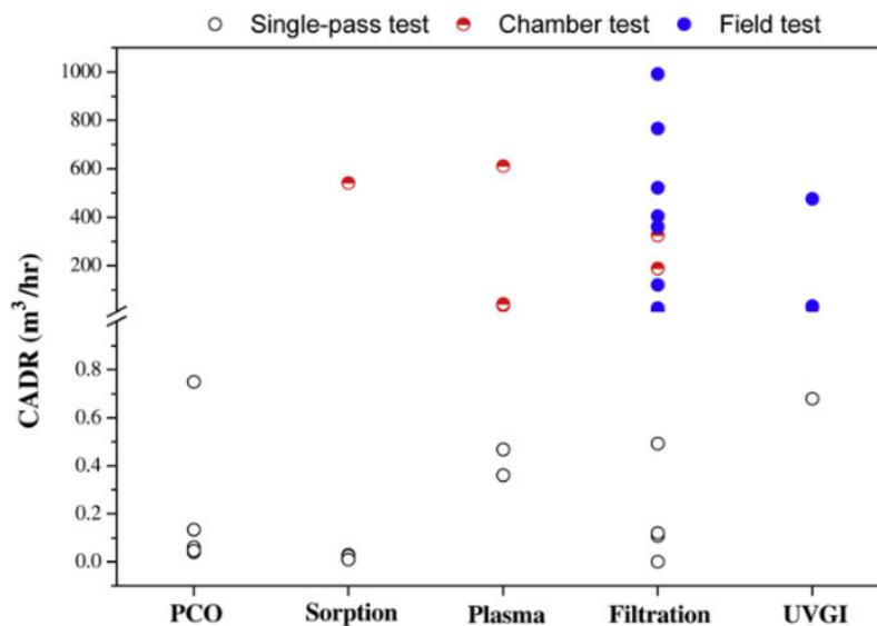
Figure 3. Summary of reported CADR  $m^3/h$ . (To convert to cfm, divide the CADR value by 1.699). UVGI refers to ultraviolet germicidal irradiation and PCO refers to photocatalytic oxidation.
